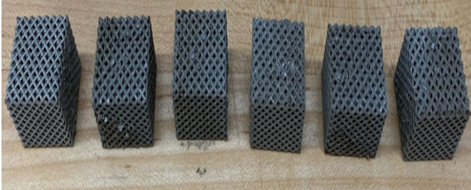
Figure 7. 3D printed scaffolds using LPBF after removal of support material and build plate.
